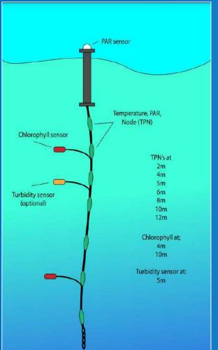
OptiCAL sensor chains relaying realtime Temperature, Chlorophyll a and PAR at 6 different depths
