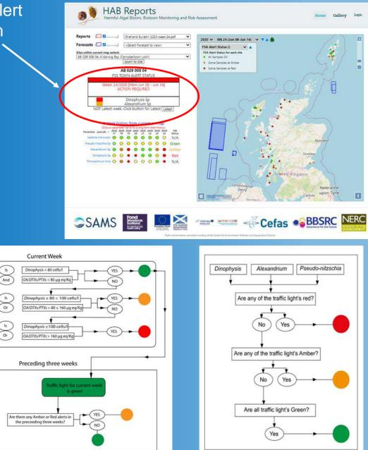
Operational Instrument - Determining the traffic light status for a site.
